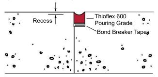
Abond breaker tape is not required in expansion joints containing polyethylene foam joint fillers. For construction or contraction joints polyethylene bond breaker tape or back-up strip must be used.
