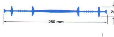
All centrally placed Supercast waterstops incorporate an eyeletted, reinforced edge flange. This enables them to be easily positioned by wiring to surrounding reinforcement.
