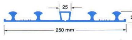
All Rearguard sections incorporate a nailing flange with a reinforced edge to provide a secure fixing that will resist tearing.
