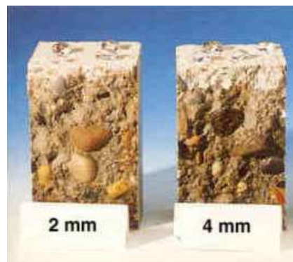
Typical penetration depth of Nitocote SN508 Creme on porous concrete. 0.25 litres/m 2 gave 2 mm penetration. 0.44 litres/m 2 gave 4 mm penetration.
