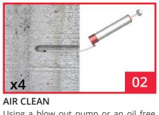
Using a blow out pump or an oil free com-pressed air lance, blow out debris from the hole four times. If the hole is wet, use air to dry it. Pay attention to changes in setting and curing times.
