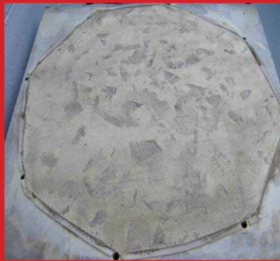
Fosroc Matacyl RB passed test, which involves 2M cycles of abrasion from ballast directly on top of the membrane
