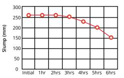
Auramix R series shows outstanding performance to keep the workable concrete for 6hrs without any delaying IST and FST.
